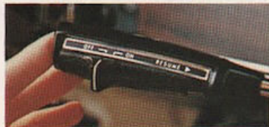
Automatic Speed Control.
