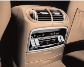
Four-zone air-conditioning system
