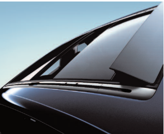
Panoramic roof system
